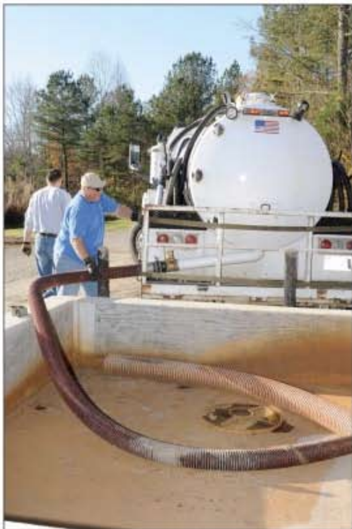
Darian Cranford handles the hose while offloading portable restroom waste at a wastewater treatment plant.
